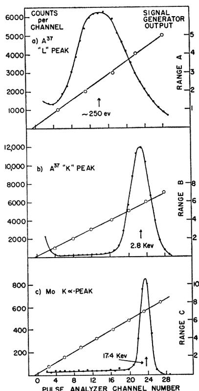
FIG. 1. Peaks produced by ~250-ev, 2.8-kev, and 17.4-kev radiations showing the decrease in percent width with increasing energy. The straight lines refer to the signal generator calibration. Precise measurements of widths, however, were made using a biased amplifier to spread the 2.8-kev and 17.4-kev peaks over many channels of the pulse analyzer.
