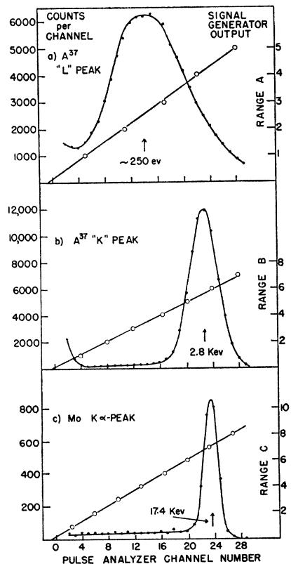
FIG. 1. Peaks produced by  $\sim 250$ -ev, 2.8-kev, and 17.4-kev radiations showing the decrease in percent width with increasing energy. The straight lines refer to the signal generator calibration. Precise measurements of widths, however, were made using a biased amplifier to spread the 2.8-kev and 17.4-kev peaks over many channels of the pulse analyzer.
