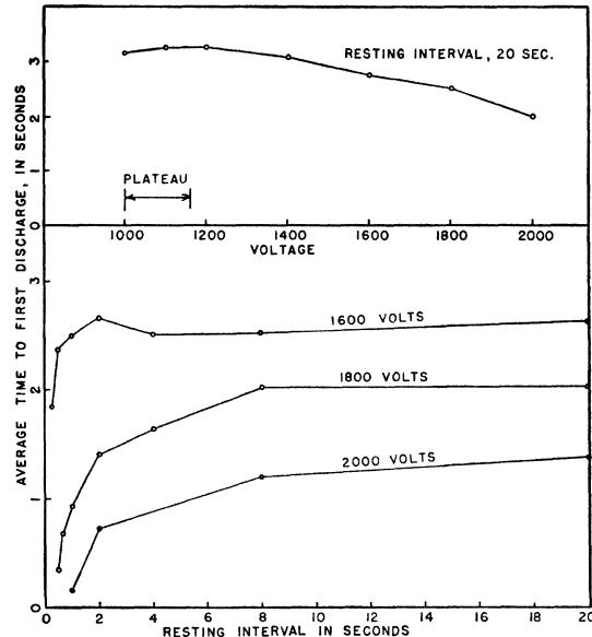
FIG. 1. Average time between raising of the voltage and the first discharge of a Geiger counter. Upper curve for constant resting period; lower curve for different resting periods and various constant voltages. Correction: The three curves in the lower part of the figure should have been labeled 1600, 2000, and 2300 volts, respectively.
