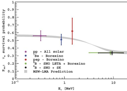
Figure 5: Electron neutrino survival probability as a function of energy. The points are the contribution of the Borexino experiment accomplished so far. The MSWLMA prediction band is the  $1\sigma$  range of the mixing parameters given in [18].
