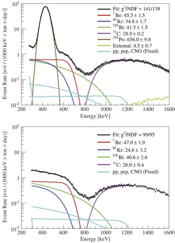
Figure 1: Two example fitted spectra; the fit results in the legends have units [counts/day·100 ton]. Top: A Monte Carlo based fit over the energy region 270–1600 keV to a spectrum from which some, but not all, of the  $\alpha$  events have been removed using a pulse shape cut. Bottom: An analytic fit over the 290–1270 keV energy region to a spectrum obtained with statistical subtraction.
