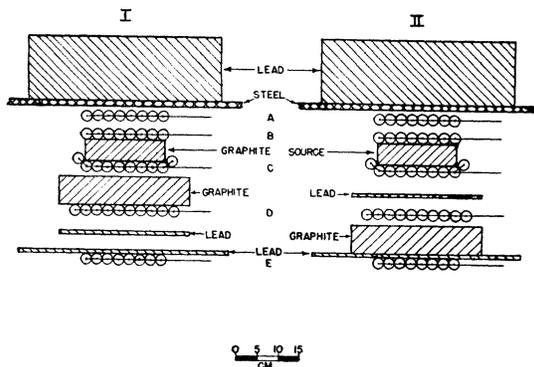
FIG. 2. Two arrangements which were alternated to compare production of bremsstrahlung in carbon (I) and lead (II). For the circuits see Fig. 1.
